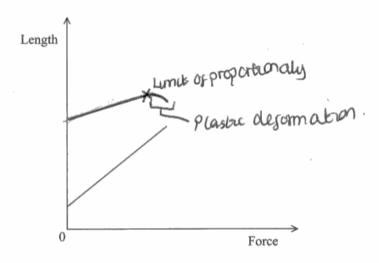
On the axes opposite sketch the graph for spring C and use it to help you describe the difference in the behaviour of springs A and C.
